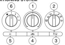
6. **Fan speed adjustment:** Controls the volume of air circulated in the vehicle.
